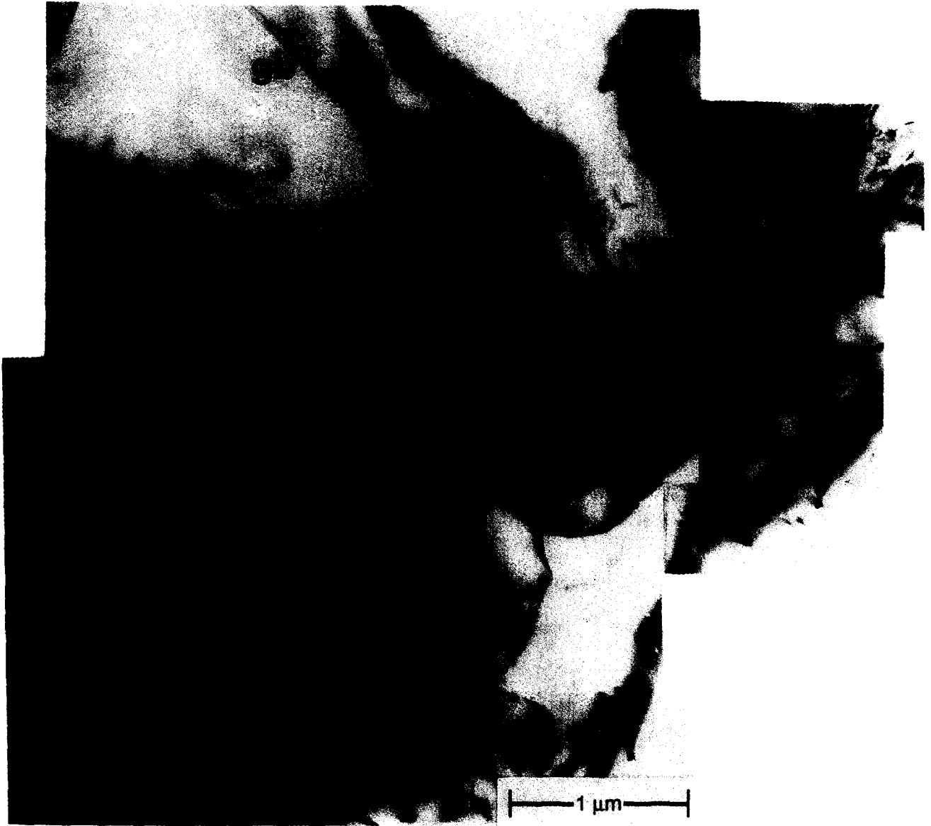
Fig. 5. Composite electron micrograph (bright field, BF) showing details of typical grain boundaries encountered. Both curved and straight grain boundaries occur. The curved boundaries (arrowed) bow towards regions of high defect densities; the region behind the curvature is virtually defect free. Note the lack of voids (bubbles) along the grain boundaries especially at triple points and at grain boundary-subgrain boundary intersections. gb : grain boundary; sgb : subgrain boundary.
