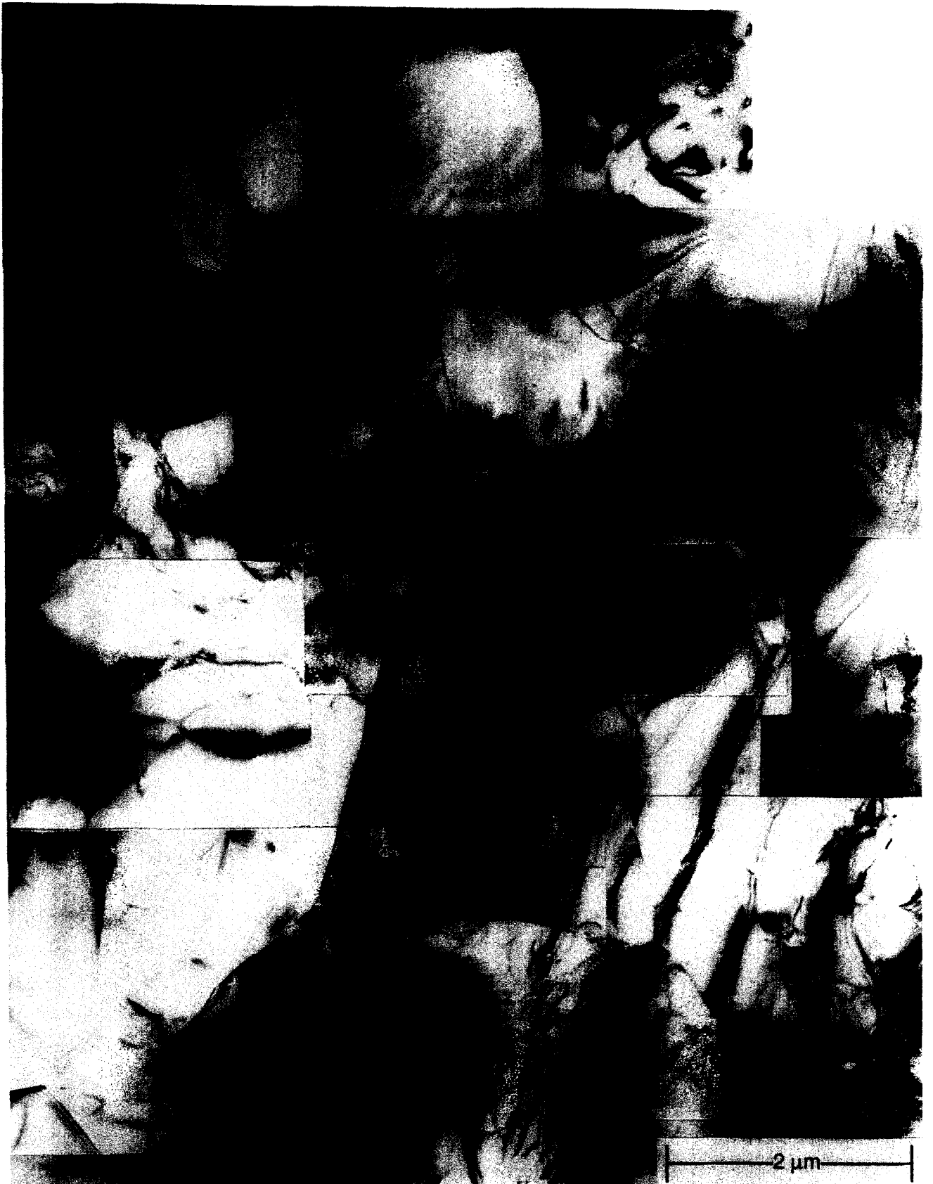
Fig. 3. Composite electron micrograph (bright field, BF) showing the microstructure of the quartz in a fine grained band. The larger grains are elongated parallel to the foliation and have well formed subgrains and high dislocation densities. The smaller grains consistently have a lower dislocation density and exhibit, if present, a disorganized cell structure. A line drawing of this area is given in Figs. 9 and 10.
